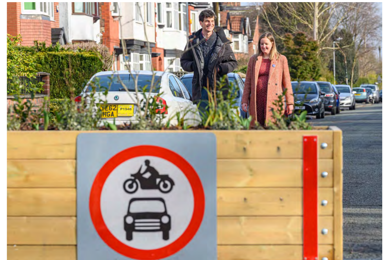
A simple modal filter in Greater Manchester. Image: Transport for Greater Manchester
