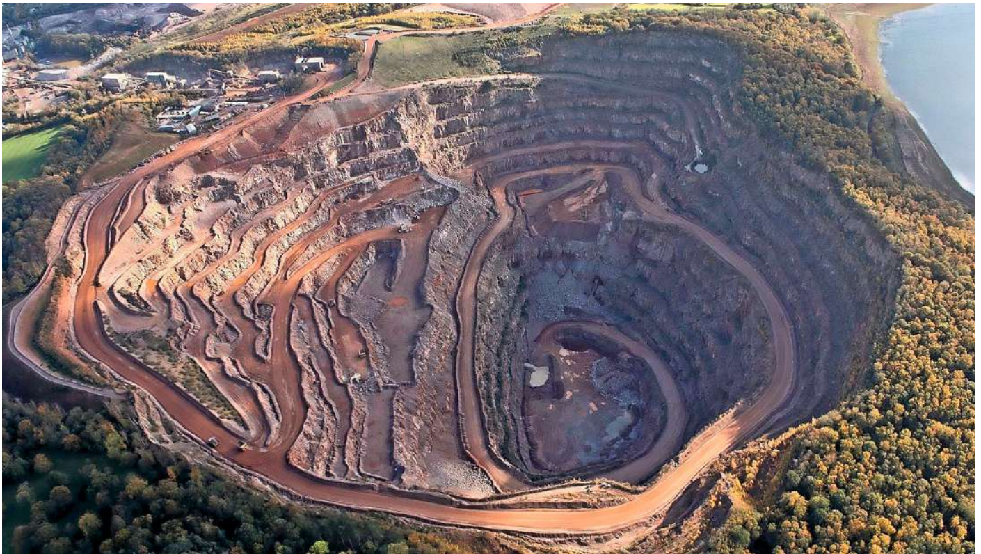
Mountsorrel Quarry in Leicestershire produces six million tonnes of granite per year and is served only by a single lead junction onto the Down Fast, meaning that a train must run in the opposite direction of travel for over a mile at 5mph. DAVID JARVIS ASSOCIATES.
