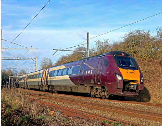
East Midlands Railway 222013 approaches Braybrooke (between Kettering and Market Harborough) with the 1012 Nottingham-St Pancras International on December 29 2022. The resilience to high temperatures of newer overhead line equipment installed on the Midland Main Line has proved markedly better than older OLE. PAUL BIGGS.
