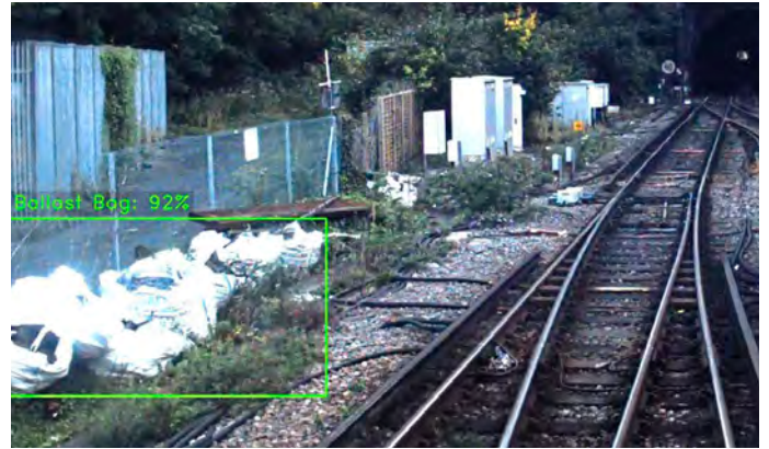
AI has recently been used by Network Rail to analysis onboard footage to identify scrap metal and materials alongside the railway. NETWORK RAIL.
