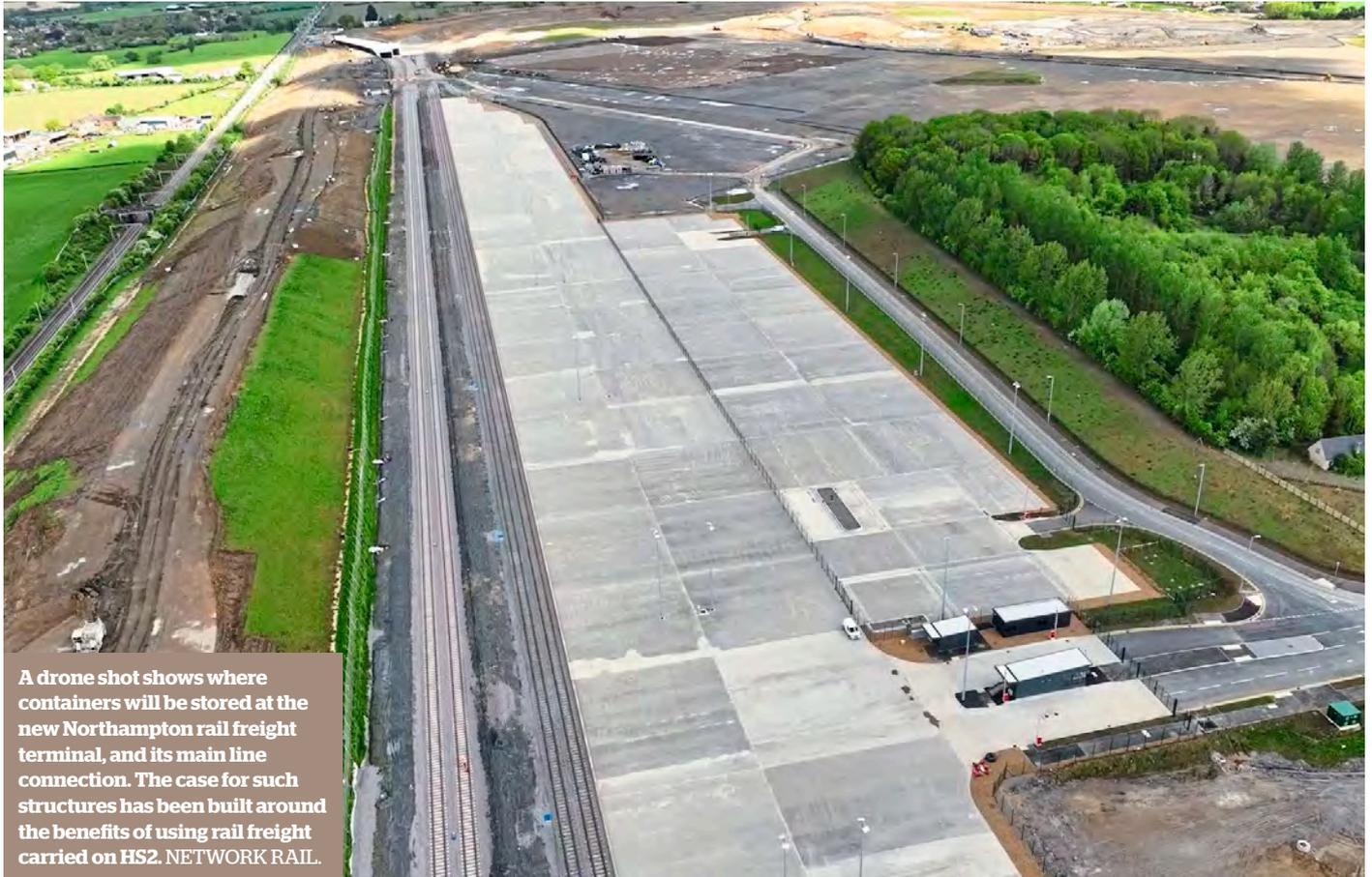
**A drone shot shows where containers will be stored at the new Northampton rail freight terminal, and its main line connection. The case for such structures has been built around the benefits of using rail freight carried on HS2. NETWORK RAIL.**
