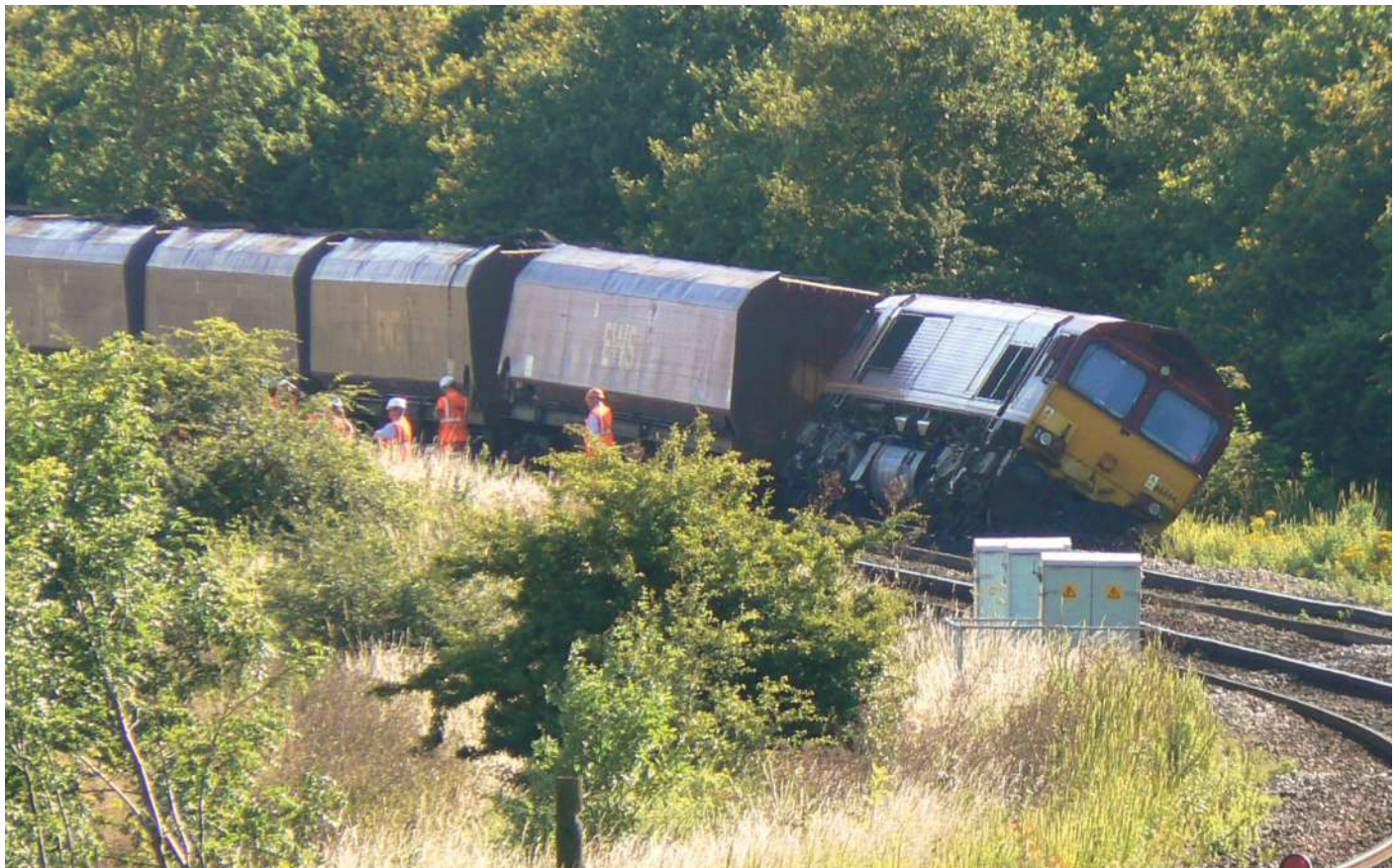
A DB Schenker Class 66 derailed between Ulceby Junction and Brocklesby Junction in Lincolnshire on the morning of July 15 2014. The '66' was hauling loaded coal wagons when a Category A SPAD (signal passed at danger) and derailment was reported and the Rail Accident Investigation Branch (RAIB) informed. Passenger and freight trains were disrupted for several hours but there were no injuries. SIMON ROBERTS.
