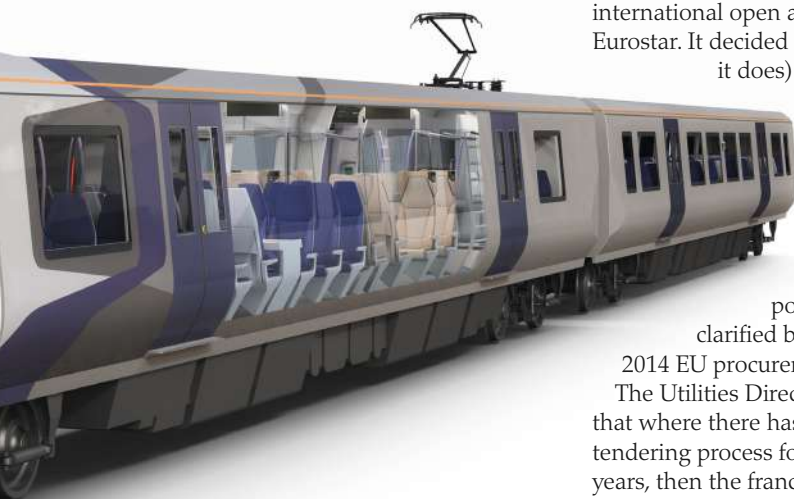
A cut-away artist's impression of an AT200 EMU designed by Hitachi for the Intercity Express Programme. Chris Jackson says procurement is a key risk that must be very carefully managed. HITACHI.
